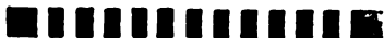
FIG. 2. A SERIES OF DOTS WHICH AT A DISTANCE OF 30 FEET LOOKS LIKE A CONTINUOUS LINE
